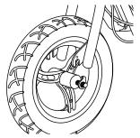
**2** Insert the wheel into the front fork with the lock washers on the outside of the fork.
